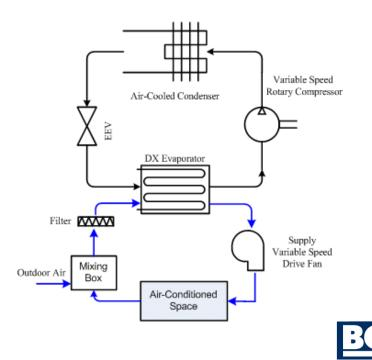
**VRF** – Supplemental for Process Loading, Complex, Expensive, Efficient
