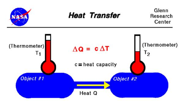
In the process of reaching thermodynamic equilibrium, heat is transferred from the warmer object to the cooler object. At thermodynamic equilibrium heat transfer is zero.
